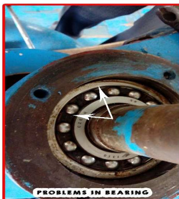
Fig.6: Wear in the Bearing
